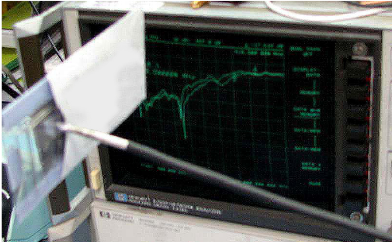
The photo above shows the portrait envelope slipped over the Design-1 RFID badge antenna to the feedline; note that the VNA now shows almost no attenuation at all.
