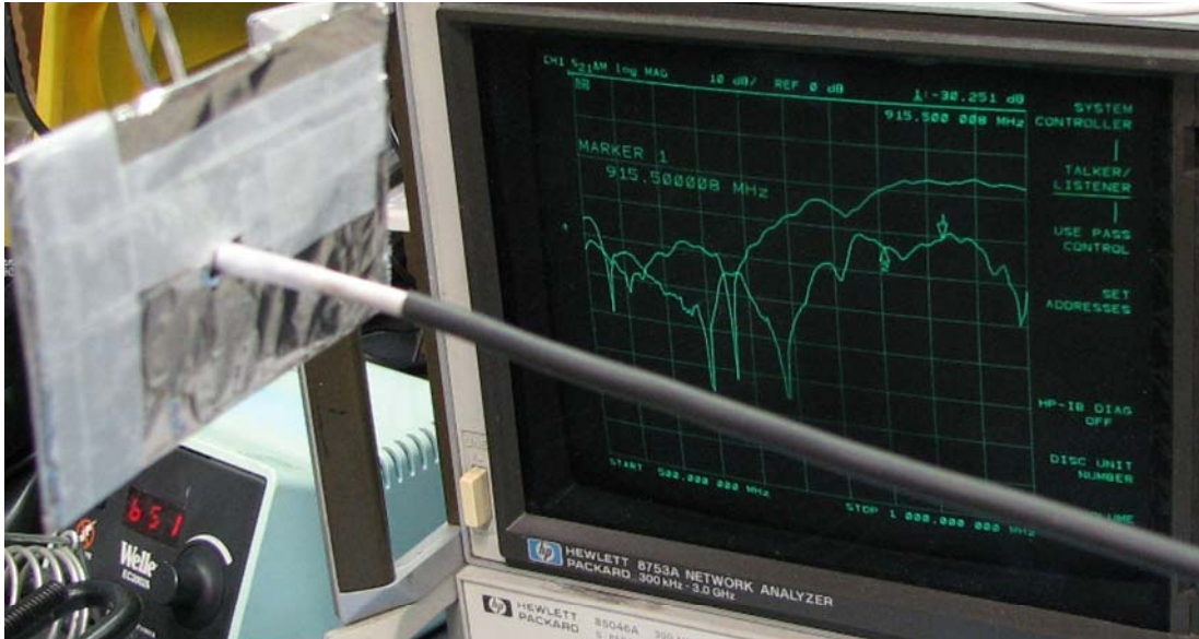
Above, the PC “badge” antenna has been entirely wrapped with aluminum foil with only the feedline protruding through a hole in the foil. Note that the transmission loss is approximately 14 dB.
