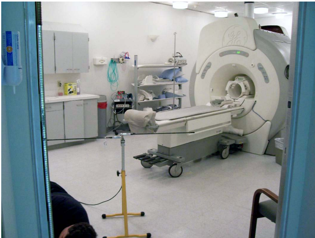
Above: Calibrated EMC Test Antenna in MRI Test Room
