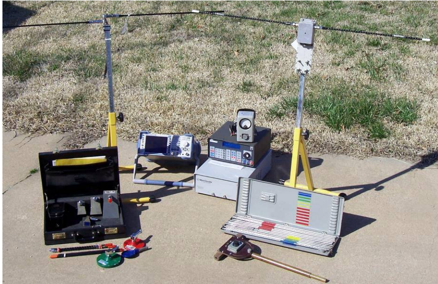
Above: Precision equipment and calibrated antennas used for MRI Room measurements
