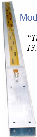
2.4 GHz 16-slot, horizontally polarized sector antenna
