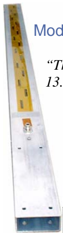
2.4 GHz 16-slot, horizontally polarized sector antenna
